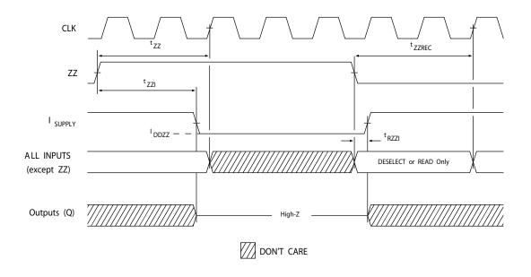
25. Device must be deselected when entering ZZ mode. See Truth Table on page 8 for all possible signal conditions to deselect the device. 26. DQs are in High Z when exiting ZZ sleep mode.
