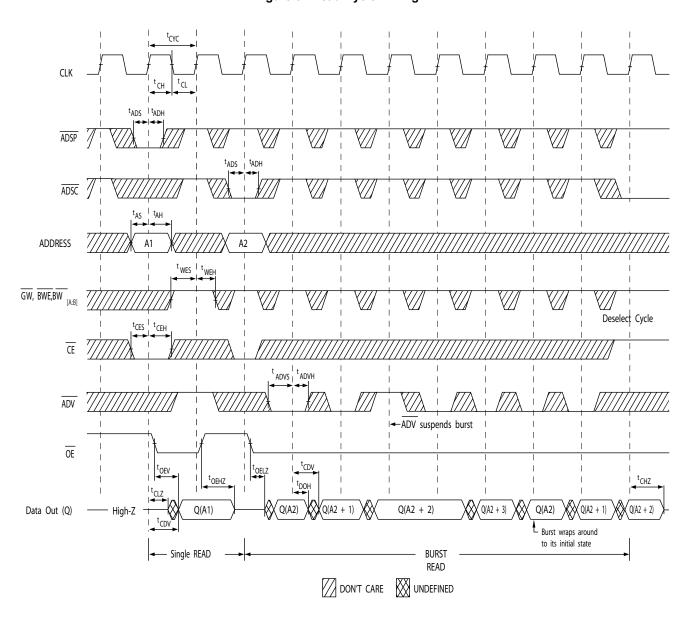
**Note** 19. On this diagram, when  $\overline{CE}$  is LOW:  $\overline{CE}_1$  is LOW,  $\overline{CE}_2$  is HIGH and  $\overline{CE}_3$  is LOW. When  $\overline{CE}$  is HIGH:  $\overline{CE}_1$  is HIGH or  $\overline{CE}_2$  is LOW or  $\overline{CE}_3$  is HIGH.
